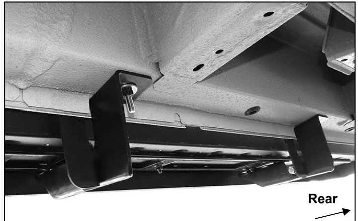
(Fig 22) Passenger side center and rear Brackets installed-mark to drill through pinch weld (For example only)
