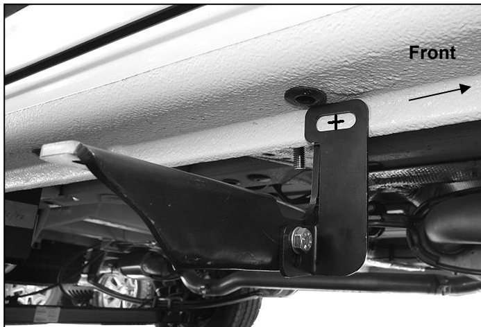
(Fig 20) Passenger side center Bracket installed
