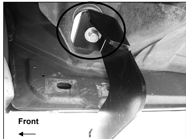
(Fig 3) Passenger/front Upper Bracket installation
