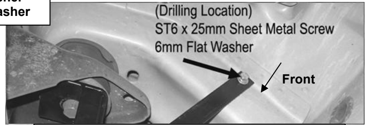
(Fig 3)Front Support Bracket(short) installation
