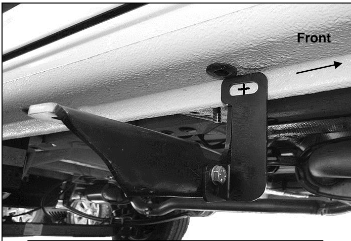
(Fig 17) Passenger side #2 Bracket installed
