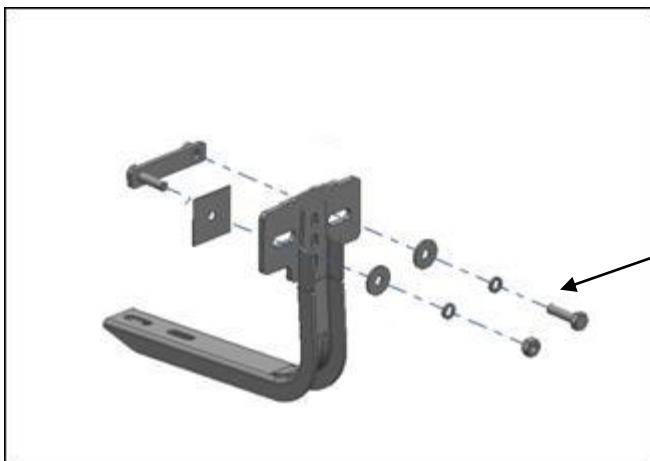
(Fig 8b) Driver Front Mounting Bracket installation
