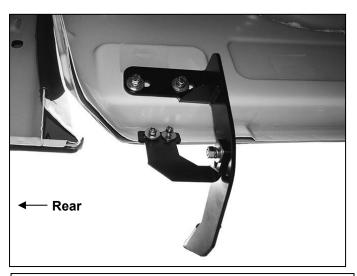
(Fig 14) Driver/Left rear Mounting Bracket assembly
