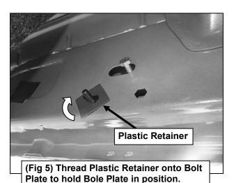
Remove Hex Bolt, rotate Bolt/Nut Plate
