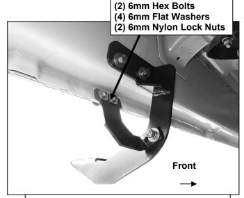
(Fig 11) Driver side front Bracket assembly
