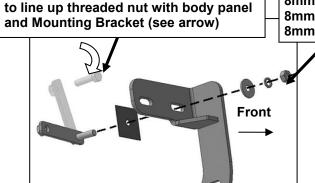
(Fig 6A) Attach Bracket to Bolt Plate
