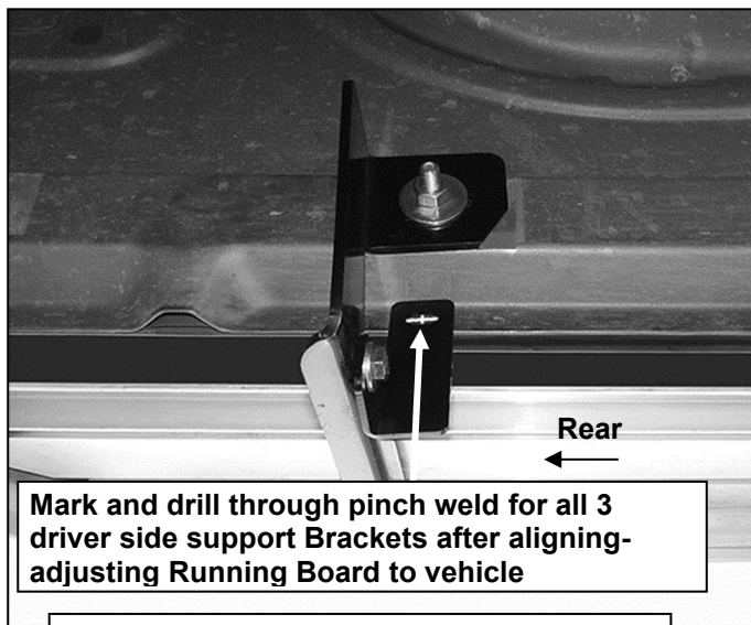
(Fig 16) Driver side rear Bracket pictured
