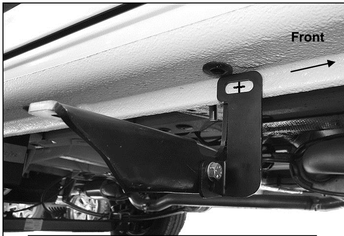
(Fig 17) Passenger side #2 Bracket installed
