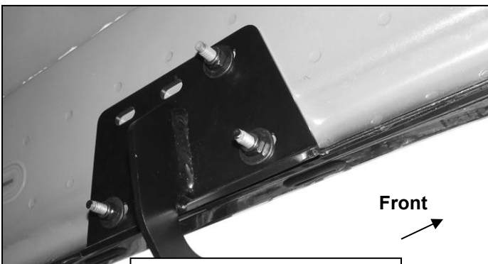
(Fig 3) Driver/left front side Mounting Bracket installed
