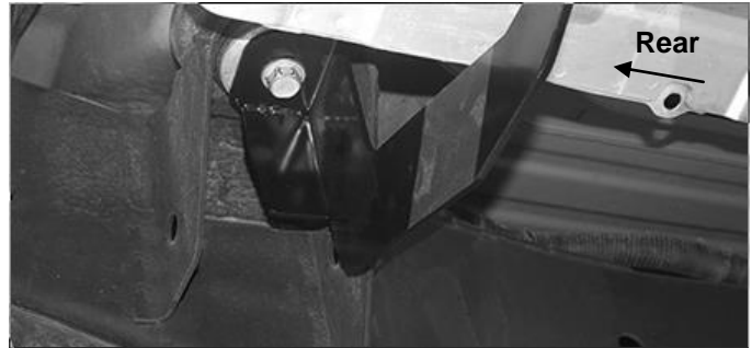
(Fig 11) Passenger side Rear Bracket Installation
