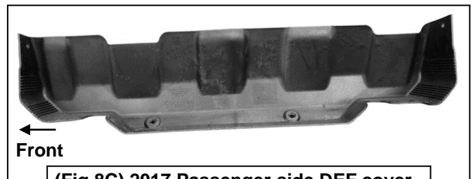
(Fig 8C) 2017 Passenger side DEF cover
