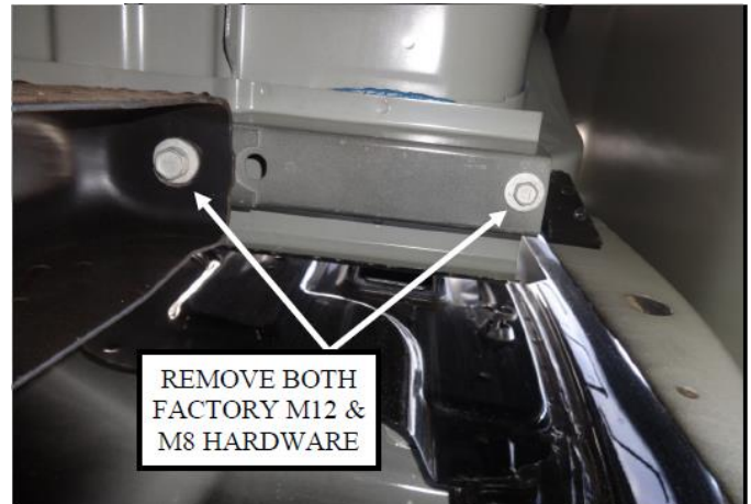
(Fig 7A) WTW Driver Rear Isolator bracket location
