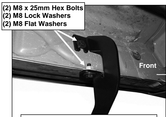
(Fig 6) Driver/left front bracket installed
