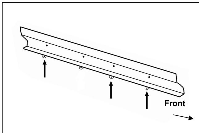
(Fig 1) Back of driver side (3) mounting locations
