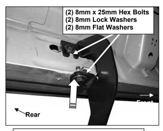
(Fig 7) Driver/left rear bracket installed
