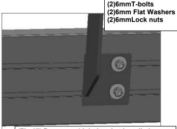
(Fig 17) Passenger/right bracket installed
