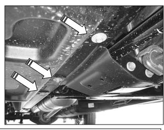
(Fig 8) Passenger side front pictured with DEF tank cover. Remove (3) hex bolts to remove cover
