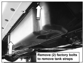
(Fig 9) Passenger side DEF tank and cover
