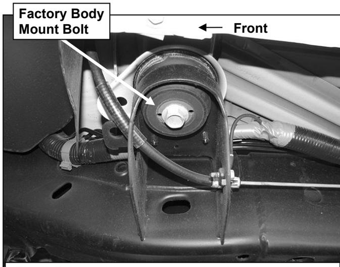
**(Fig 1) Driver side front mounting bracket pictured**
