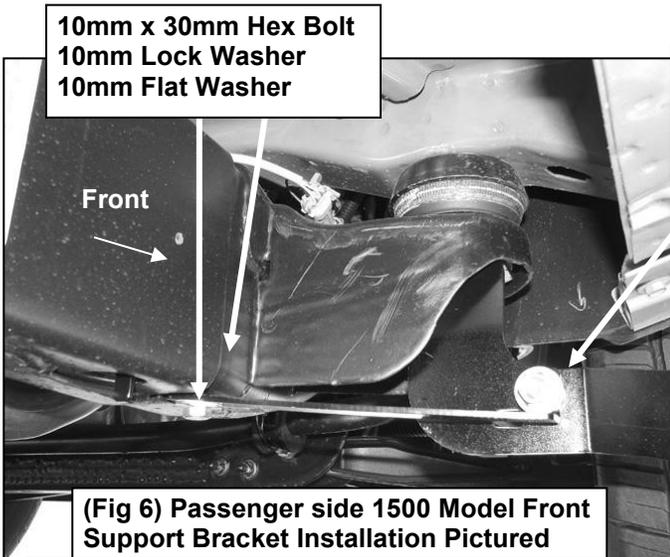
(Fig 6) Passenger side 1500 Model Front Support Bracket Installation Pictured
