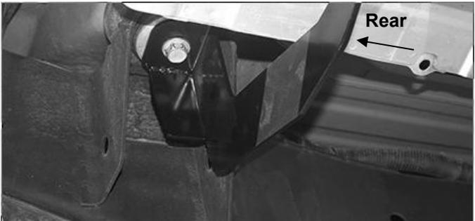
(Fig 9) Passenger side Rear Bracket Installation
