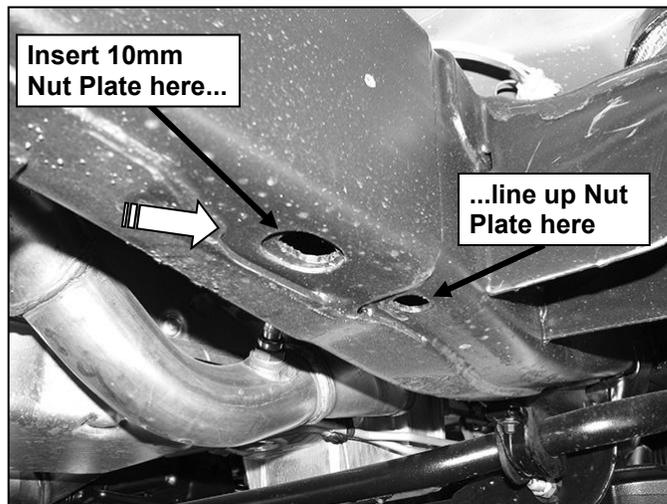
(Fig 4) Bottom of frame on passenger side
