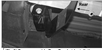
(Fig 9) Passenger side Rear Bracket Installation
