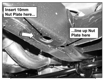
(Fig 4) Bottom of frame on passenger side
