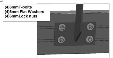
(Fig 11) Passenger side Bracket Installation
