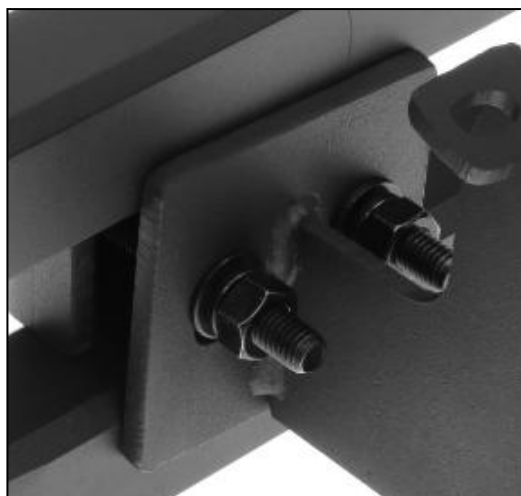
(Fig 19) Driver/Left side bracket installed
