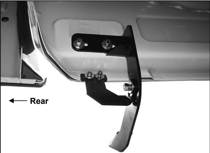
(Fig 16) Driver/Left rear Mounting Bracket assembly
