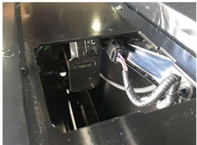
10. Install grille to vehicle. Connect TSS harness.
