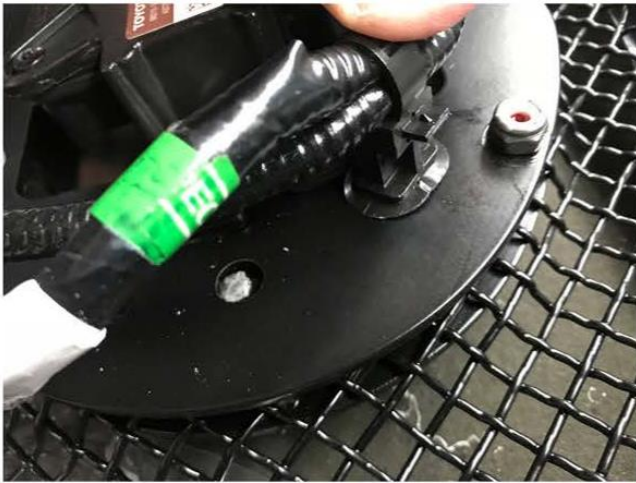
7. Install complete assembly to mounting studs with spacers in place. Use (4) #10 lock nuts and Torque to 30 in- lbs. Note orientation of TOP side of module. Connect harness to module, press harness cable mounts into position as shown.
