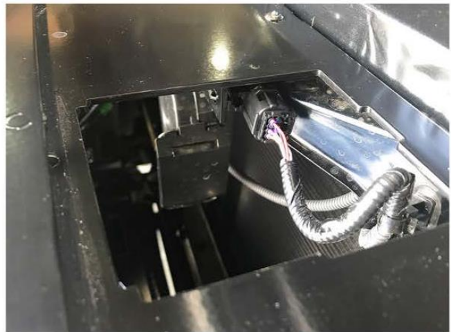
10. Install grille to vehicle. Connect TSS harness.
