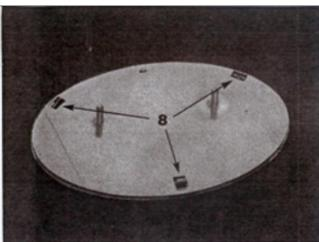
Trim the factory tabs protruding from the back of the emblem plate prior to installatin onto the mesh grille to keep the tabs from contacting the mesh.
