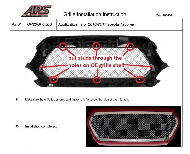
The instruction here is for your reference only. You may need to bend the grille a little bit to adjust to fit. We strongly recommend the professional installer for best result. We are not responsible for any damage caused by the installation. Thank you for choosing our product!
