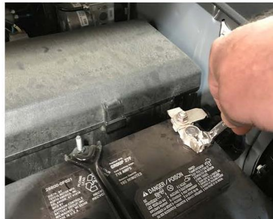
12. Reconnect negative battery terminal.
