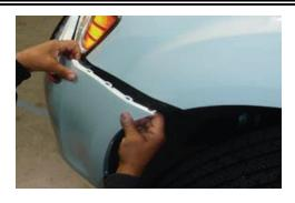
Step 2-5: Pull side fender outward to unclip.
