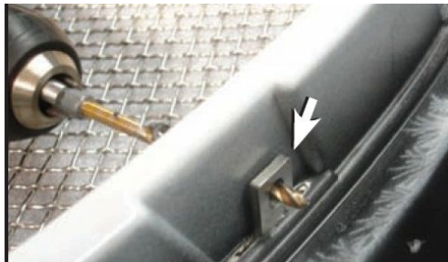
Step4-4:Drill a 3/16 Hole through the Brackets on the side and bottom of the Mesh Grill.
