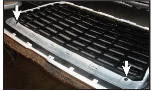
Step3-2:Remove 2 Screws on the corners of the Grille Shell.
