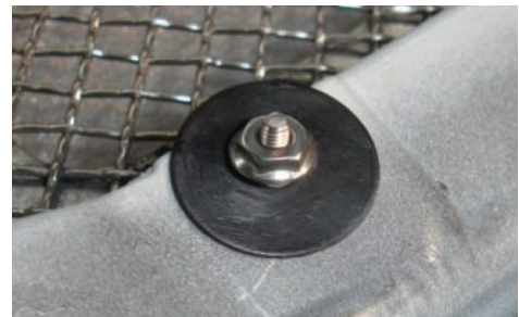
Step4-3:Insert Fender Flat washers along the top of the Screws on the mesh Grille,Tight with Lock Nuts.
