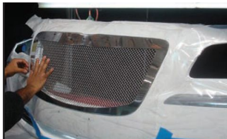
Step4-3:Place Mesh Grille over the Factory Grille Shell.
