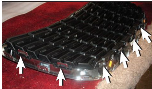
Step4-1:Unclip the Factory Grille from around the Chrome Frame.
