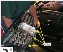
Center the billet insert in the opening. The top mounting tabs should align with factory mounting holes (it may be necessary to slightly bend the brackets). Hold the billet insert firmly in place. Make sure it is centered. Mark the holes in the lower mounting tabs to the opening. Remove the billet insert and drill a 1/8"hole at each mark.
