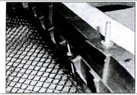
Place the shell with the billet grille back onto the vehicle, and secure using the factory hardware. Tighten down all hardware.
