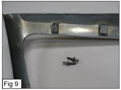
Thread a stud in each nut welded to the grille. Center the grille into the opening. Slide the L brackets on the mounting studs; the longer L 10 brackets install on each end. Secure the brackets with the flat washers and K-Lock nuts.
