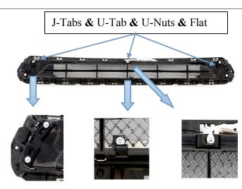
Make sure the billet grille is centered and tighten the fasteners.
