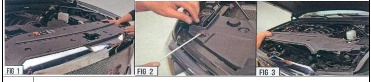
Begin by removing the plastic core support cover shroud. There will a number of plastic "Push Tabs" that secure the cover.
