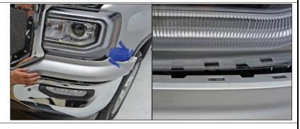
Put Core Support Cover back into place and fasten down with plastic push tabs that were removed prior. Re-Install all hardware that was removed in step #4.
