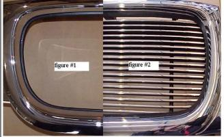
The instruction here is for your reference only. You may need to bend the billet grille bars or tabs a little bit to adjust to fit. We strongly recommend the professional installer for best result.
