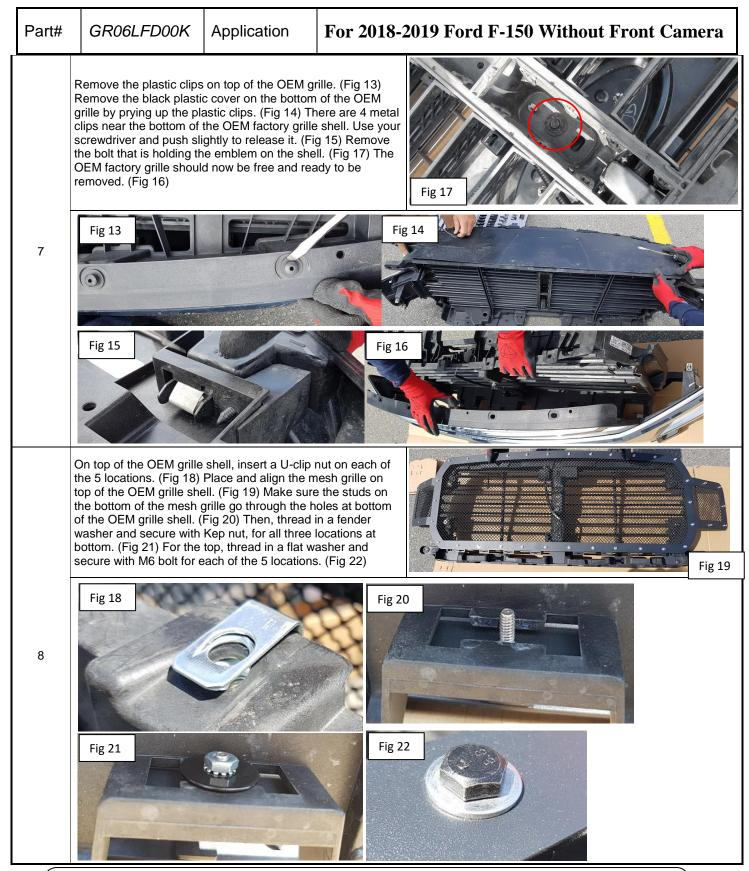
The instruction here is for your reference only. You may need to bend the billet grille bars or tabs a little bit to adjust to fit. We strongly recommend the professional installer for best result. Please use masking tape and tape the OEM grille shell along the edge to protect your vehicle during installation. We are not responsible for any damage caused by the installation. Thank you for choosing our product!
