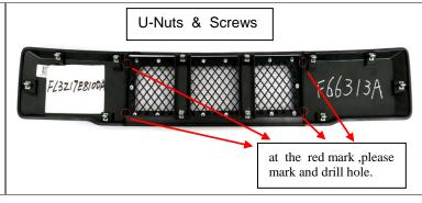
Make sure the grille is centered and tighten the fasteners, but do not over-tighten.
