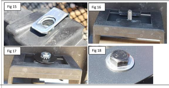
Put the grille back to the truck. Plug in the sensor plugs and fix wiring with clip. Re-install the fender lip and black plastic cover using the stock screws and clips. At this point you want to look over your work and examine the gap alignments around all edges and in between the new grille and the vehicle components and body lines. Carefully close the hood for a complete visual inspection. If adjustment is needed, you can loosen the top mounts and shift side to side even gaps.
