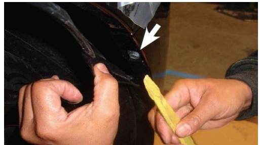
Step2-4: Use a Plastic Prybar to separate the Fender Cover from Bumper Shell and remove 10mm Bolt.
