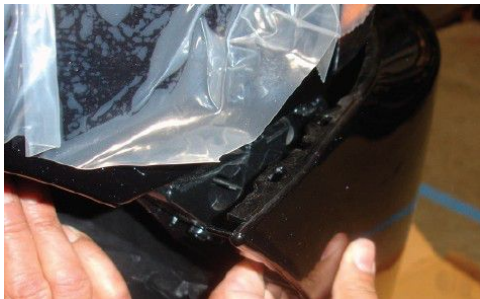
Step2-5: On each end, Clips secure the side bumper. Carefully pull the side bumper outward to release clips.
