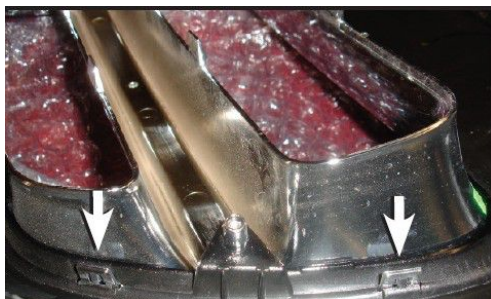
Step3-5:Unclip 8 Clips from around the OEM Grille Shell and remove (OEM Grille Shell will come out from front).
