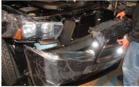
Step2-7:Remove factory grille and bumper (grille and bumper are connected together)
