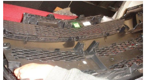
Step3-4: Remove Factory Grille.
