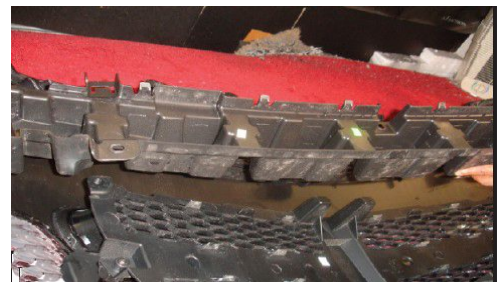
Step3-2:Remove Bumper Support.
