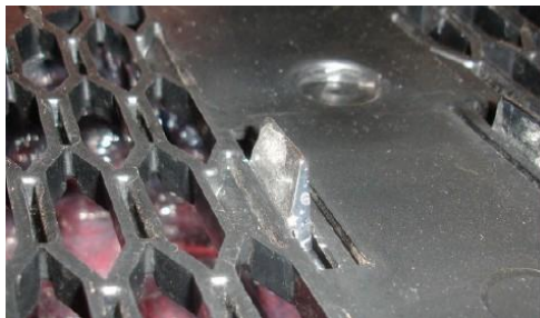
Step3-3:Unclip 16 clips from around the Factory Grille.
