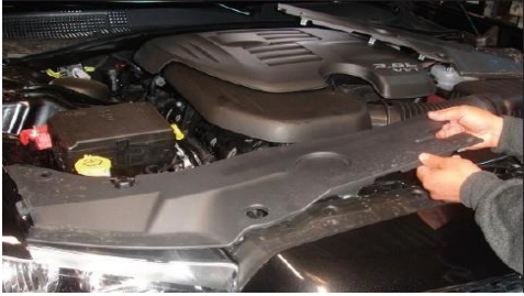
Step2-1: Pop hood, Remove 2 Plastic Covers above the Factory Grille Shell.
