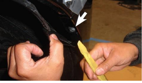
Step2-1: Remove 4 Clips along the Factory Grille Shell.
