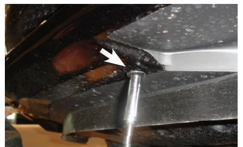
Step2-4: Use a Plastic Prybar to separate the Fender Cover from Bumper Shell and remove 10mm Bolt.
