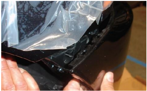
Step2-5:On each end,Clips secure the side bumper,Carefully pull the side bumper outward to release clips.
