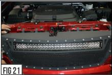
Reverse the bumper removal order process to re-install vehicle components. Start by inserting the (6) screws across the top that hangs and secures top grille frame. **SEE FIG 22-23.**
