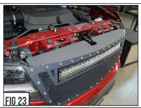
Push back into place the front bumper fascia so that the plastic body will meet and sit flush with the front fenders and hug the edge of the head lamps.
