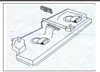
A portion of material must be cut from the core support to mount the headlamps. Use this diagram on the left to cut the area needed to recess the headlights. Make your cut as indicated by the shaded areas.
