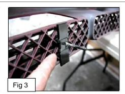
Make sure the billet grille is centered and tighten the fasteners, but do not over-tighten.
