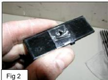
Secure billet grille using the 'J' hook Tab from the back side of the OEM grille shell.(Fig 2&3)
