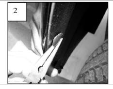
Pull the inner fender wells away from the bumper cover. This will gain access to disconnect the turn signals lights and fog lights. Use a slotted screwdriver to unfasten the light covers; twist the lights from the sockets to disconnect them (3). Once the lights have been disconnected; remove the bumper cover assembly (4).
