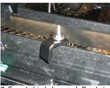
7. From behind place an L-Bracket on the threaded studs on the mesh grille and tighten with provided 6-32 Lock Nuts.
