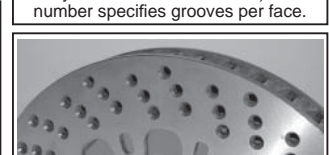
D & SD = Cross Drilled. (Drilled holes chamfered). Still preferred with some pad materials but can compromise disc life.
