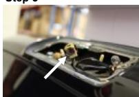
Remove the brake light bulb out of its socket
