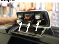
Remove the third brake light by disconnecting the brake light bulb and the two reverse light bulb sockets out of the third brake light housing
