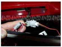
Step 6: When connecting our new Anzo third brake light make sure orange wire lines up with the white/yellow wire and black to red/green wire
