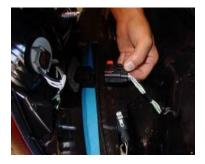
Step 3: pull off the tail light from the car and unplug the wire harness.
