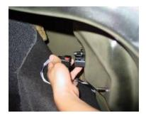
Step 6: Once light is on the car plug the wire harness into the light and then screw the three locking screws in.
