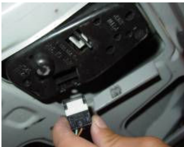
Step 3: Pull the cover down to expose the tail light cover and plug the wire harness.
