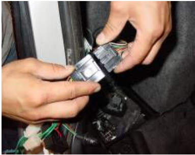
Step 13: Plug the new tail light wire harness in to the original wire harness.
