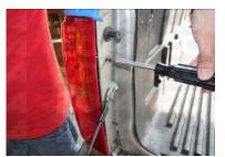
Step 3: Use the phillips screwdriver to remove the two screws holding in the tail light.
