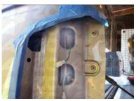
Step 6: Peel off the protective cover from the resistors and place in the two holes onto the frame of the body.
