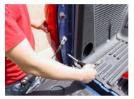
Step 2; Remove the upper and lower screws
