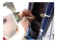
Step 8: Connect the resistor to the taillight housing.
