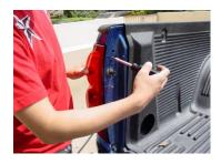
Step 1: Lower the tail gate exposing the two screws.
