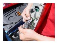
Step 7: Connect the pigtails to the stock sockets.
