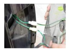
Step 7: plug the two resisters into the tail light.
