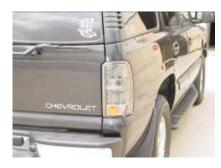
Step 8: Put the tail light in and screw in the two screws to hold the tail light in place.
