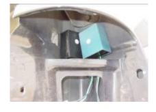
Step 6: Remove the protective sticker backing from the resisters and stick them inside the top tail light housing.
