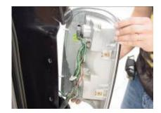
Step 5: Remove the tail light from the vehicle.
