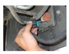
Step 2: Unplug the middle wire harness from the circuit board.
