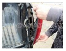
Step 2: Pull the tail light off from the vehicle.
